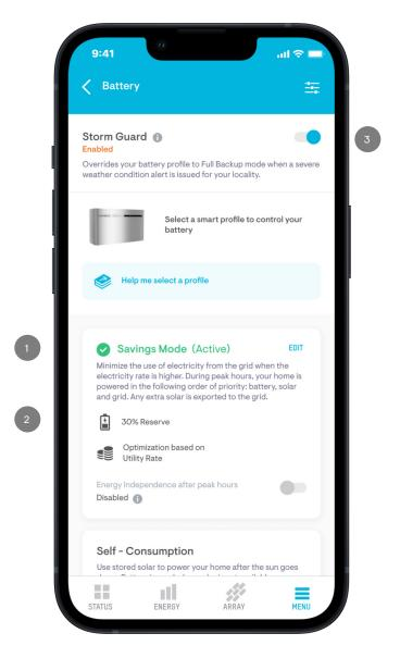
To complete the Savings mode configuration, you must have access to the electric rate schedule details of your utility account. You must also decide how much of your IQ Battery capacity is held in reserve for backup power in case of a grid outage. This is referred to as your reserve capacity.
